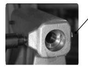
**Note**. Do **not** adjust the screws at the side of the tailstock as these are factory set.
