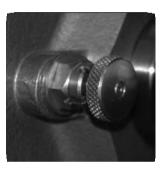
**Item 7 - Indexing Pin** To engage the indexing pin rotate the head of the pin 90° until it slides inwards, then rotate the handbrake wheel (item 6) until the pin engages preventing the spindle fromrotating. To disengage pull out the pin and rotate the head 90°.
