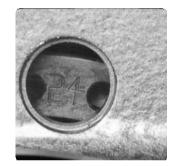
**Item 8 - Index Viewing Glass** All lathes have 24 indexing holes in the back of the spindle, which are used for indexing and locking the spindle. Each hole represents 15 degrees for indexing purposes.
