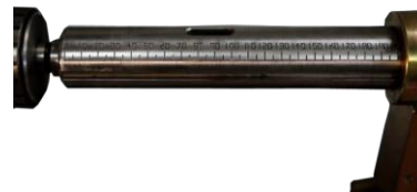
Total Spindle Extension 215mm
