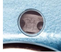
24 machined holes on headstock pulley for indexing and spindle locking
