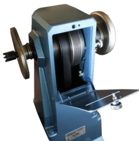
Easy to open hinged headstock door
