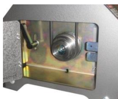
Access door for easy adjusting of belt on motor pulley
