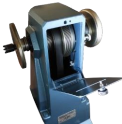
Indexing pin and Spindle Lock with Hinged Headstock door
