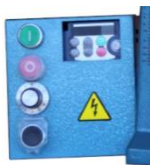
Electronic Variable Speed with digital display located on moveable switch box
