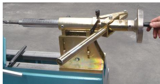
Fine adjustment up to 105mm extension
