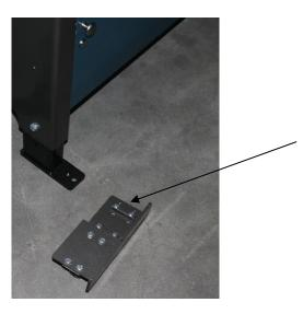
2. Insert the lifter under the stand so that the pivoting plate rests against the bottom of the tray. You may need to adjust the height of the lifter arm. To do this do you simply adjust the bolt hole position.
