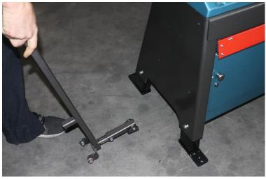
3. Press down on the lifting arm so that the stand lifts into the air and place on the two fixed wheel feet.
