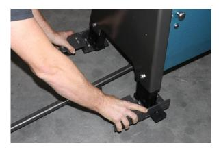
4. Lower the lathe by lifting the arm.
