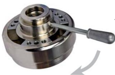
Chuck removal using the tommy bar
