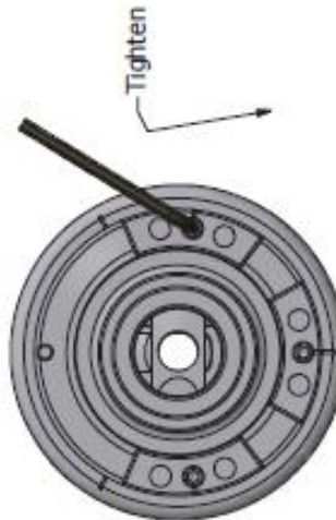
Move weights to desired position and retighten
