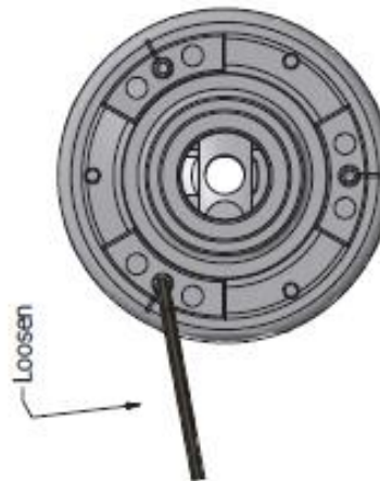
Insert 4mm Allen Key and loosen screw to adjust
