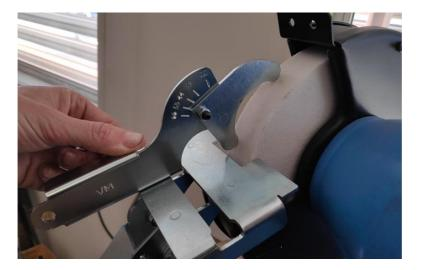
The Grinding Rest Quick Tool Setter can be used to set and grind other popular angles of 22°, 33°, 44°, 55°, 66° & 80°. To set the desired angle, place the Grinding Rest tool setter (as shown) flat on the Grinding Rest and adjust until both radii are touching the wheel.
