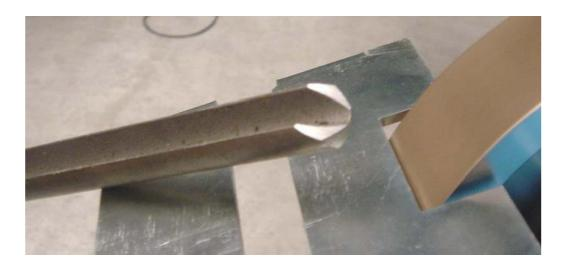
4. **Important:** Make sure that the tool does not get too hot and change colour (brown or blue) as this will reduce the hardness of the metal and shorten the life of the tool. To prevent this, make sure you periodically dip the tool in water. If you find the tool heating up too quickly then you may need to re-dress your wheel or apply less pressure on the grinding wheel.
