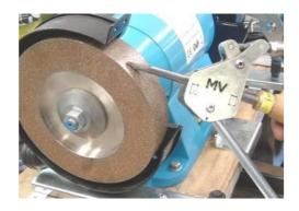
Flat profile spindle gouges - 33°
